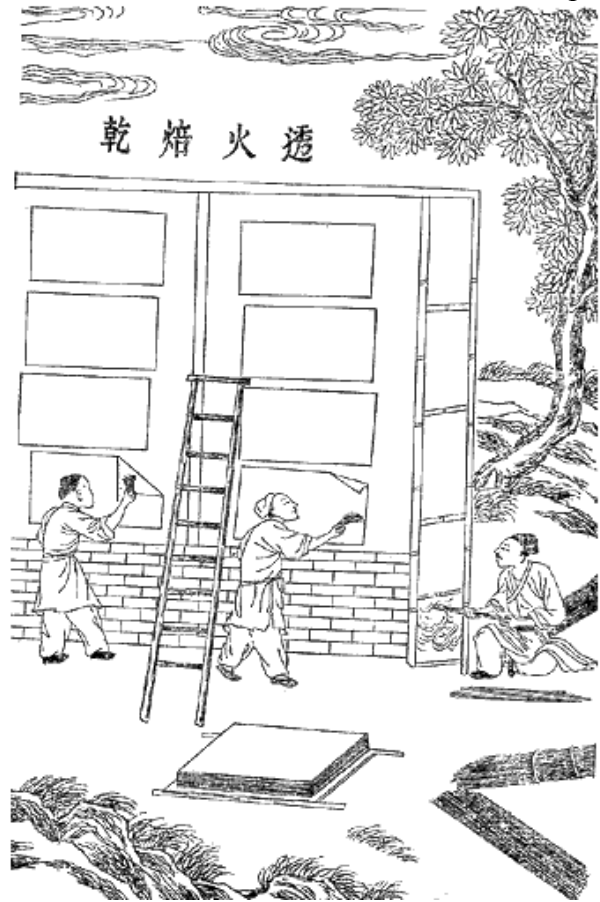
Paper was one of ancient China’s major gifts to the world, invented during the Han dynasty in the early 2nd Century CE or earlier. Here, papermakers post freshly-made sheets to dry.
