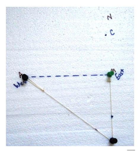
9. Change places with the ends of the string on the East-West line segment,  $\overline{AM}$ . Repeat steps 7 and 8 to construct the other two corners of the square.
